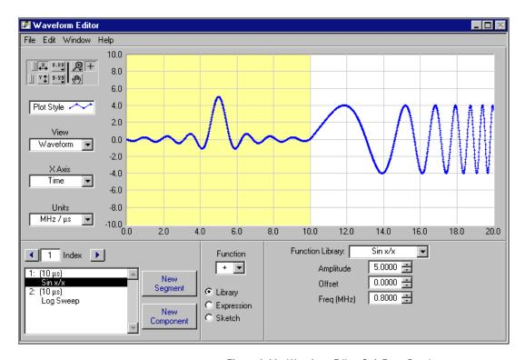
Figure 1-11. Waveform Editor Soft Front Panel
